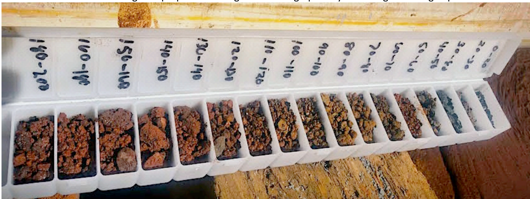
Above: circulation mud containing cuttings comes to the surface (left) and it is filtered for cutting collection (right) Below: cuttings are prepared and organized stratigraphically according to drilling depth
