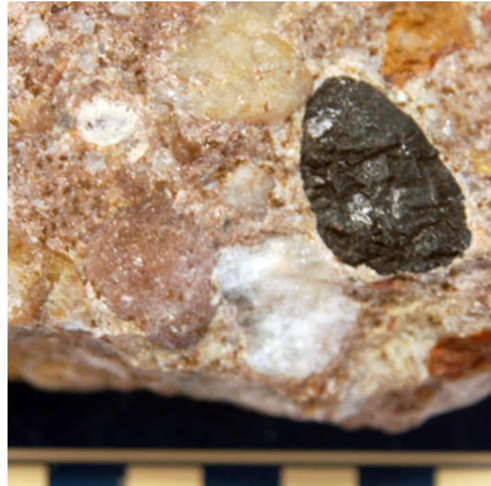
Rounded grains of gravel are cemented in this clastic sedimentary rock called conglomerate
