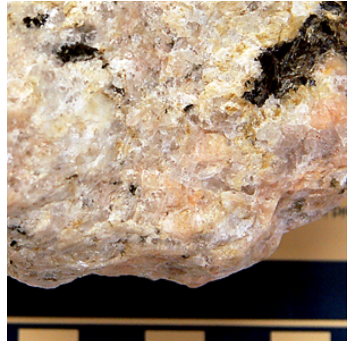
Interlocking crystals in a pegmatitic granite (intrusive igneous rock)
